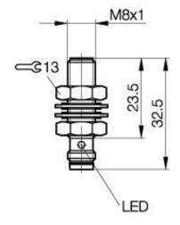
Inductive Sensors BES 515-324-E5-C-S 49 M8x1 x 32,5 normally-open Sn=1,5mm shielded
